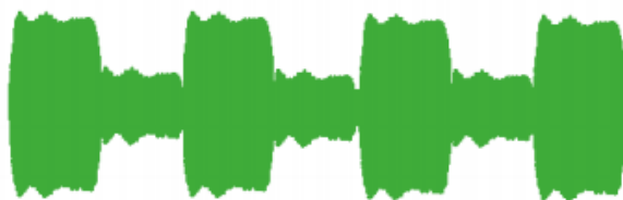
Fig. A - HF Response Showing Overshoot and Ringing
