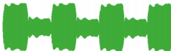
Fig. B - HF Response Corrected to Reduce Overshoot and Ringing
